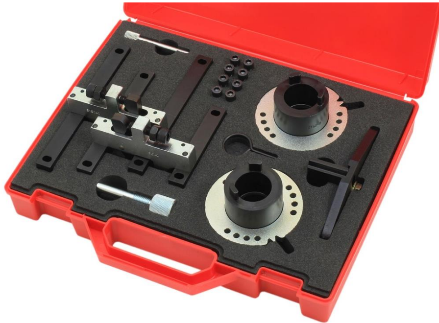
7468-10506 – GAT5150 – Petrol engine Setting / Locking Tool kit
